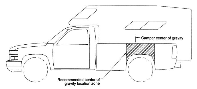
Any accessories or other equipment added to this vehicle after final date of manufacture must be weighed or have their weight determined, and the weight deducted from the prescribed Cargo Weight Rating (CWR) of this vehicle. This extra weight may shorten the center of gravity zone of the vehicle.
