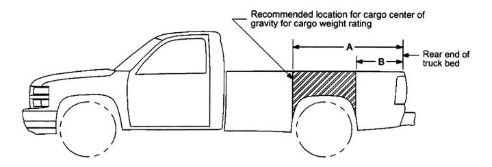
Use the rear edge of the load floor for measurement purposes. The recommended location for the cargo center of gravity is at point C for the CWR. It is the point where the mass of the body is concentrated and, if suspended at that point, would balance the front and rear.
