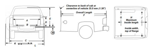
Important notes: D = Top of bed floor to top of bed rail E = Top of bed floor to top of Cab K = For dual rear wheels 2 or 4 wheel drive L = Includes quarter panel flare width © = Top of bed floor to top of bumper equals 86.36 mm (3.4") for both short and long box
